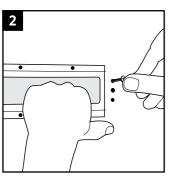
Fix the back plate with the two screws.
