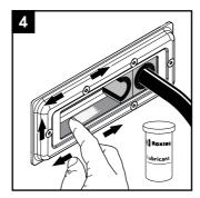
Lubricate the exposed packing space
